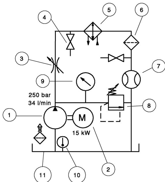
**Fig. 1** The pilot-scale water hydraulic system. 1 Pump, 2 motor, 3 restrictor valve, 4 gate valve/sampling, 5 heat exchanger, 6 filter, 7 flow meter, 8 pressure regulator, 9 pressure meter, 10 thermometer, 11 vented reservoir
